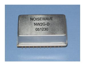
NoiseWave announces the immediate availability of the NW-2GD Dual-In-Line packaged amplified noise model. The unit features broadband frequency coverage from 10 MHz to 2 GHz. Power out is -5 dBm and the spectral flatness is +/- 2.0 dB. The unit operates with +15 Vdc and draws 100 mA.
